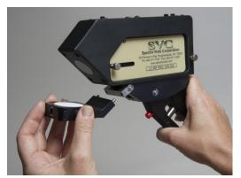
The leaf clip assembly is quickly attached or removed when switching from the Leaf Clip mode to the Contact Probe mode. The assembly is secured to either the Spring Actuator or to the parking dock with neodymium magnets.
