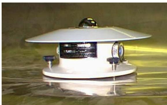
Precision Infrared Radiometer
